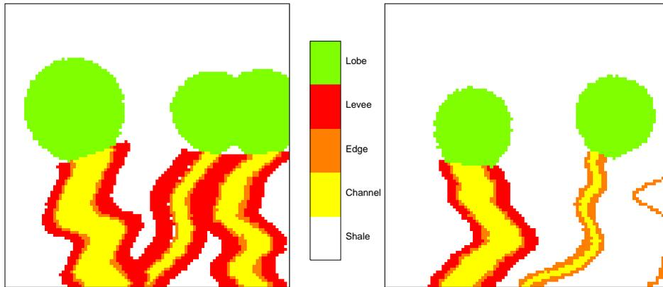
Figure 10: Horizontal slices through a `lobesim` model with lobes of constant size and levee sands associated to the channels. The proportions of channel, lobe, and levee sand were 0.1, 0.1, and 0.05, respectively.
