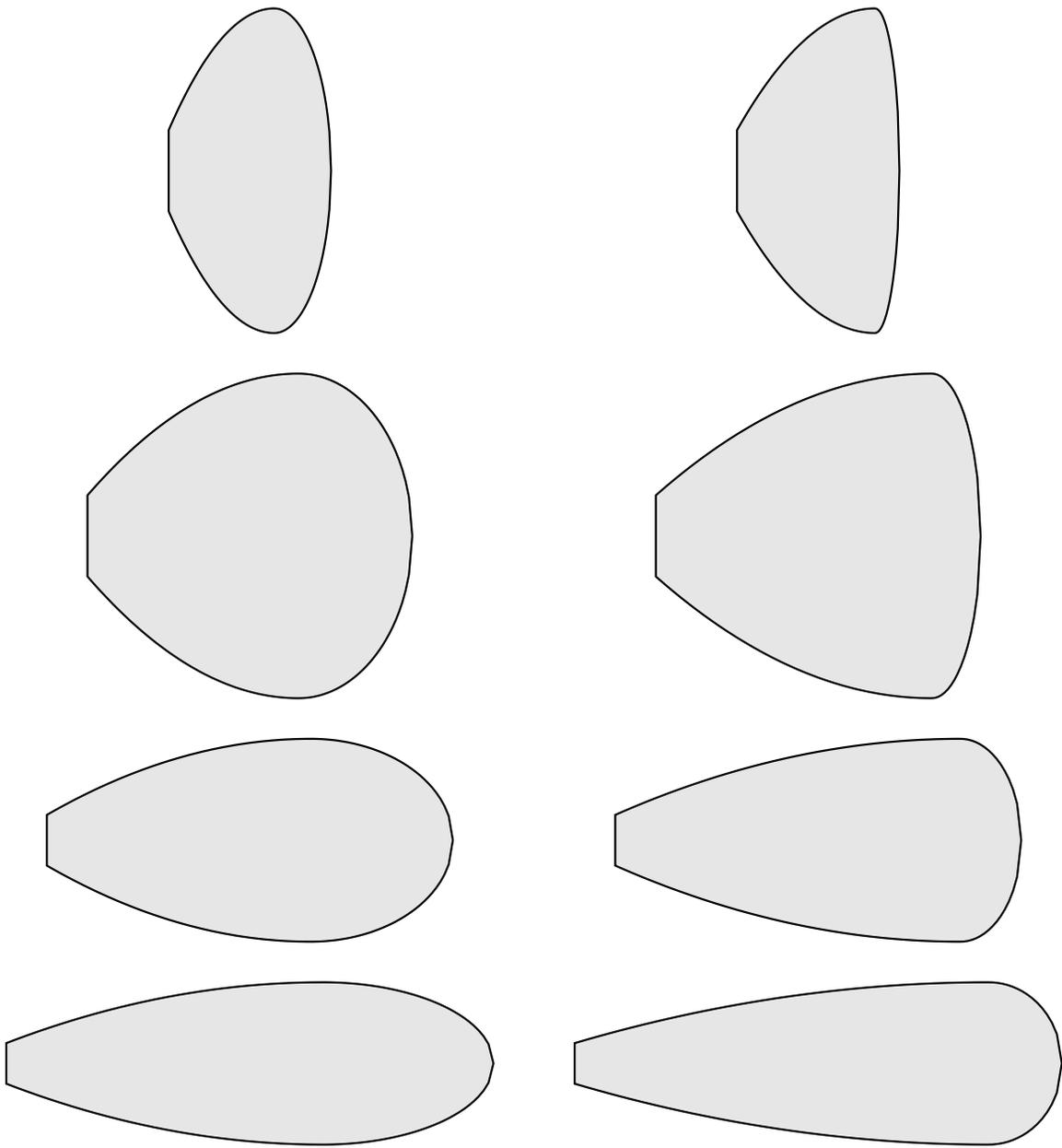
Figure 2: Example lobe geometries for various parameters. From top to bottom the width / length ratio decreases from 2.0:1 to 1:1 to 0.5:1 to 0.33:1. The relative position of the maximum width is 0.65 on the left and 0.85 on the right.
