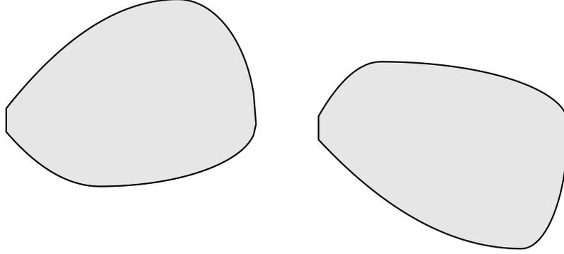
Figure 4: Two asymmetric lobe geometries. The lobe shape and first derivative are continuous around the lobe.
