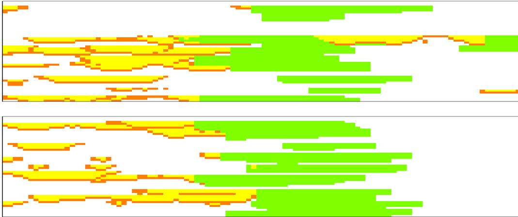
Figure 9: Vertical slices through a `lobesim` model with lobes of constant size. The target proportions of channel and lobe sand are both 0.2 in this case.
