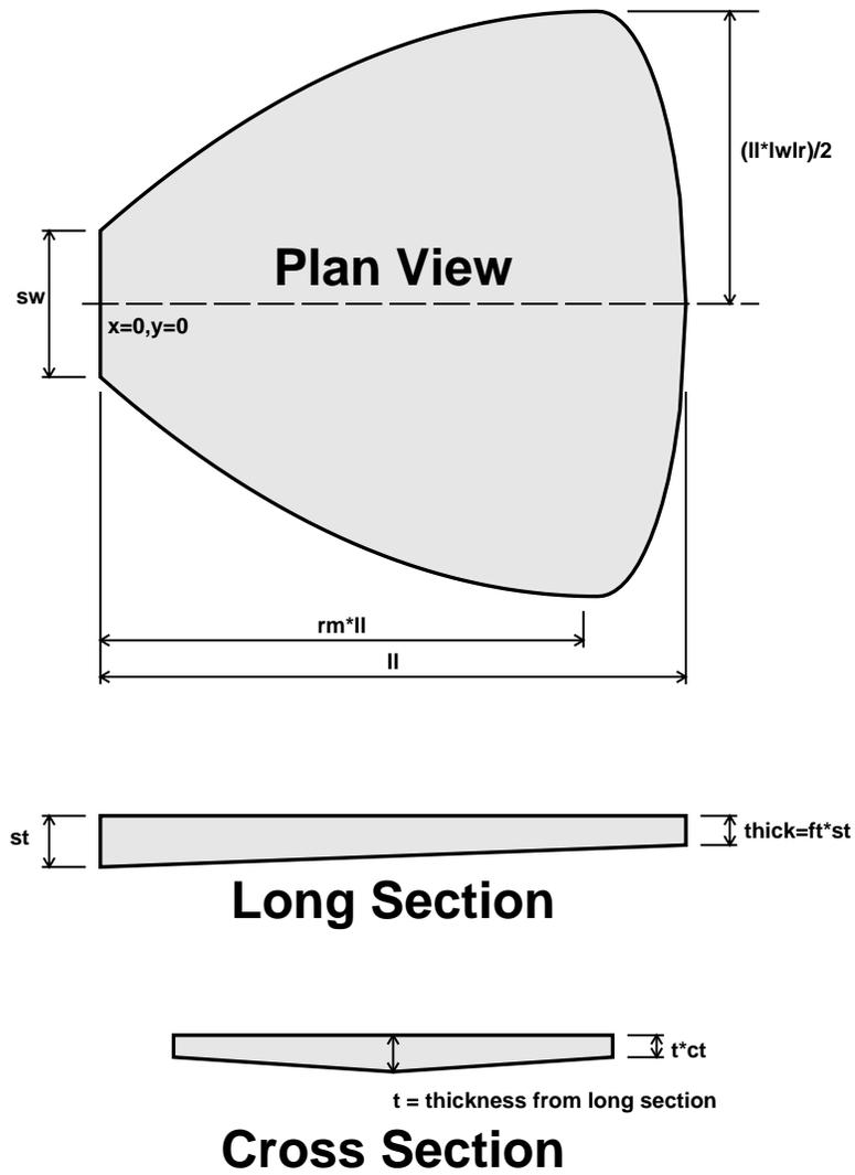
Figure 1: Parameters needed to describe the 3-D lobe geometry.
