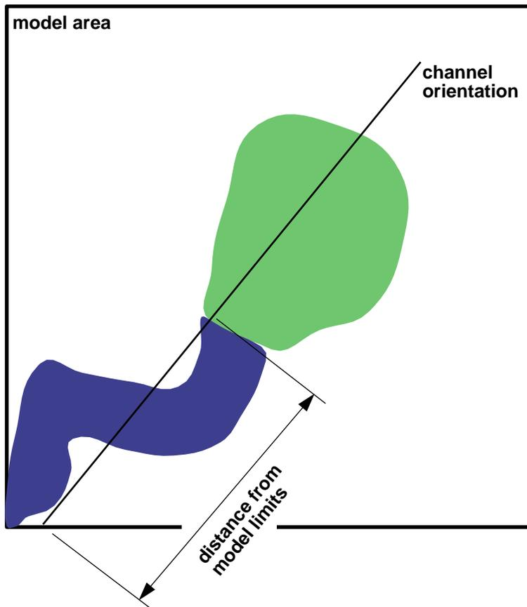
Figure 5: Lobes could be positioned with the same orientation as the associated channel. The only positioning parameter is then the distance from the model boundary.
