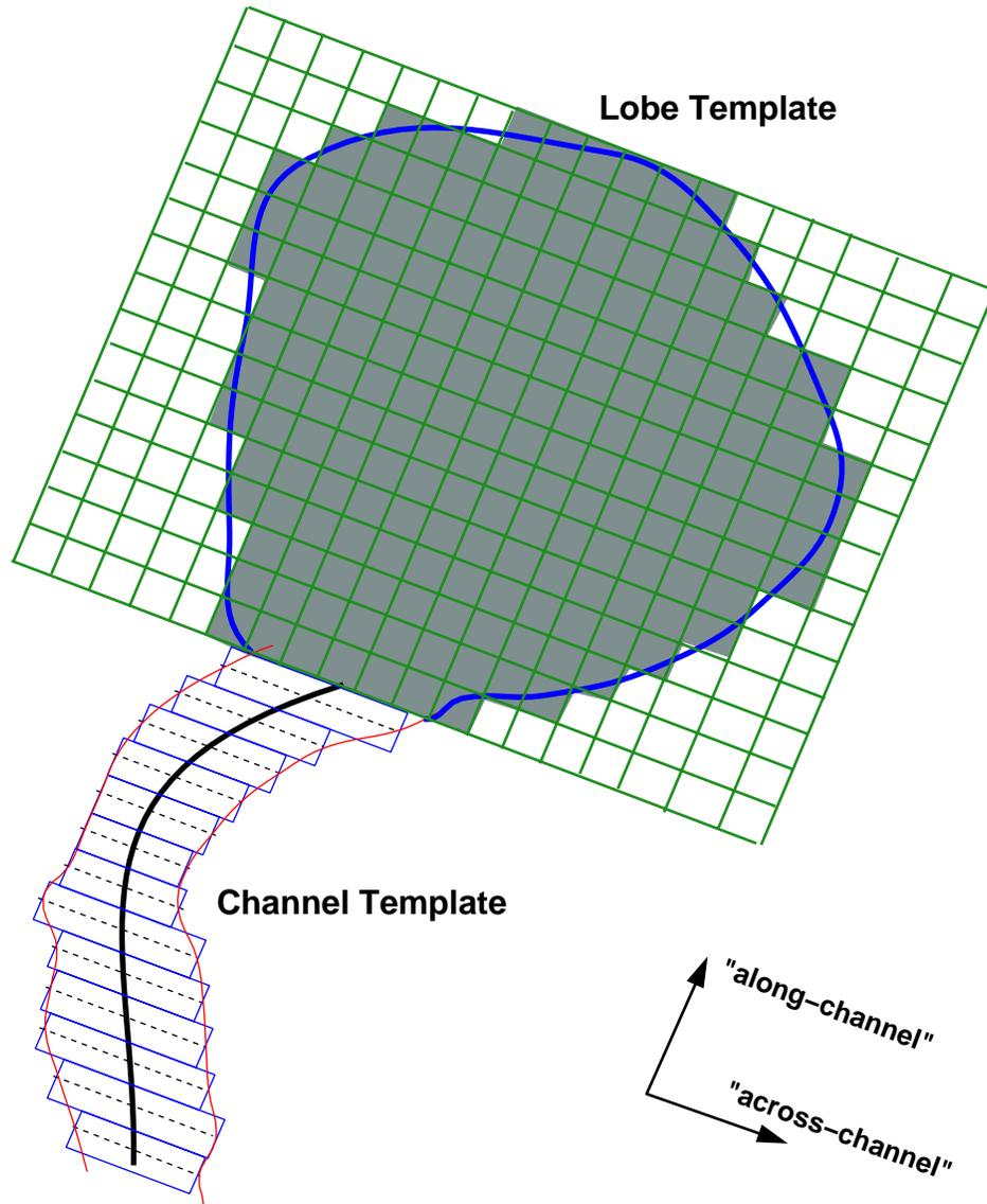
Figure 6: Channels and lobes are represented by templates. In the case of lobes, the gray shaded area is kept in memory together with the depth under each cell.
