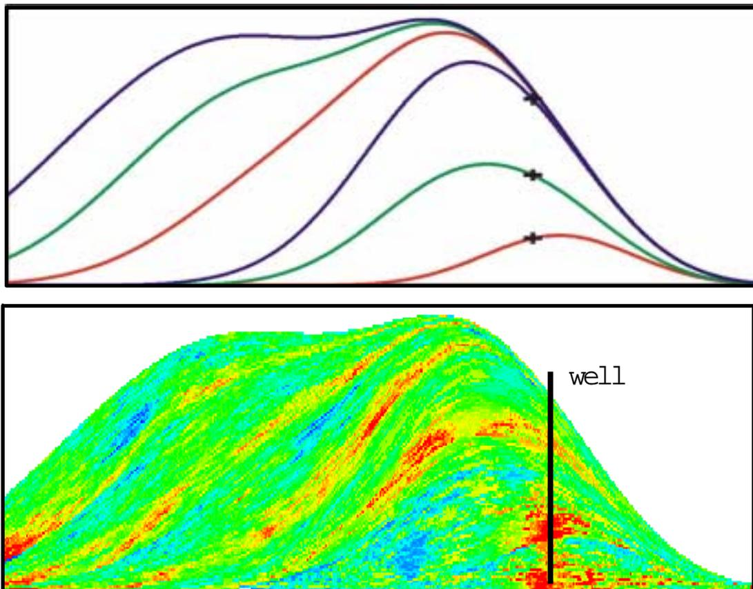
Figure 23: Simulation of the Wandoo. Top: Surfaces generated with “backstepping” rule, but constrained to three intersections in Well 6. Bottom: Trend simulation constrained by sediment units and well log.
