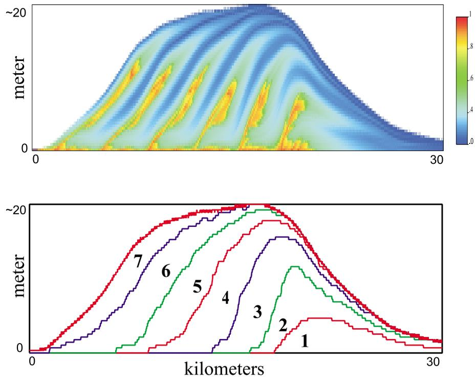
Figure 9: Top: Sand distribution derived from Sedflux “analog” for the Wandoo field and surfaces extracted along the sediment unit boundaries.
