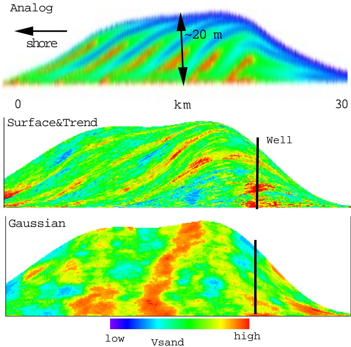
Figure 2: A. Sedflux “analog”. B. Sand fraction simulation constrained to the surface-geometry and trends using method presented in this report. C: A “conventional” gaussian simulation using the variogram model from Figure 1.
