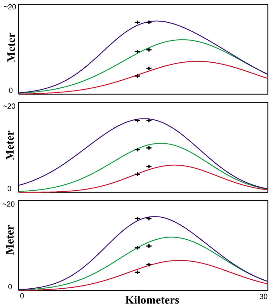
Figure 20: Three realizations of surface models from `Surfsim` conditioned to Wandoo well 6 and Wandoo well 3 (Well 3 is downdip).
