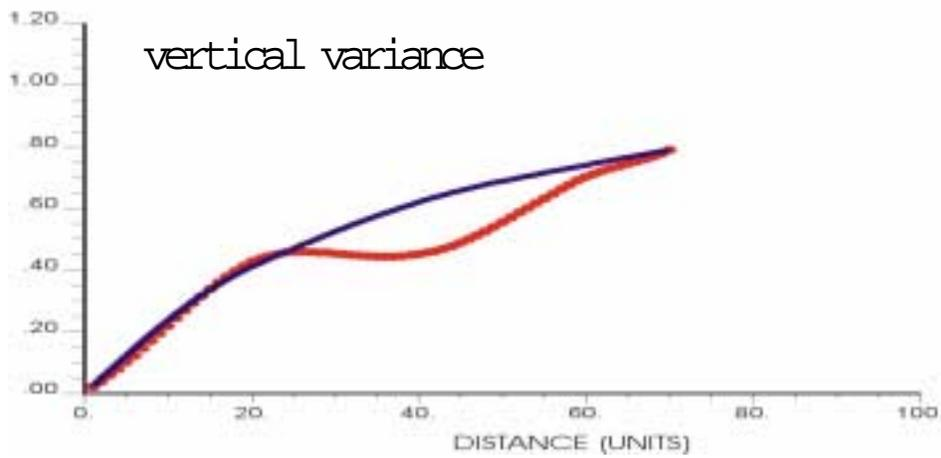
Figure 1: Sedflux “analog” for the Wandoo field and variograms of the fraction sand (red-data; black-model).
