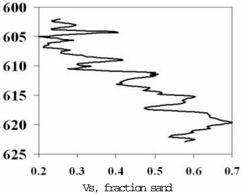
Figure 19: Log motifs for Wandoo Wells 6 and 3 (fraction sand derived from gamma ray). (See [7] for formation interval picks.)
