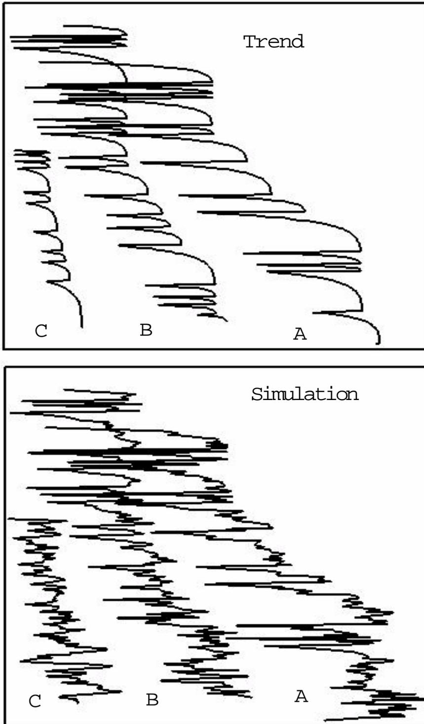
Figure 8: Sample log motifs comparing the sand distributions of trend template with trend simulation from three vertical sample locations (see Figure 7)
