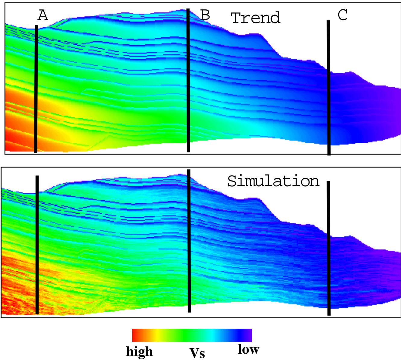
Figure 7: Trend template with nested vertical and horizontal sand distribution compared with trend simulation sand distribution.
