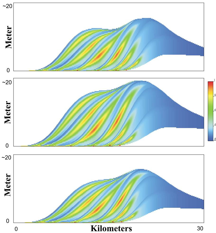
Figure 18: Trend models after building in the trend *templates* into the sediment units of unconditional surface models.
