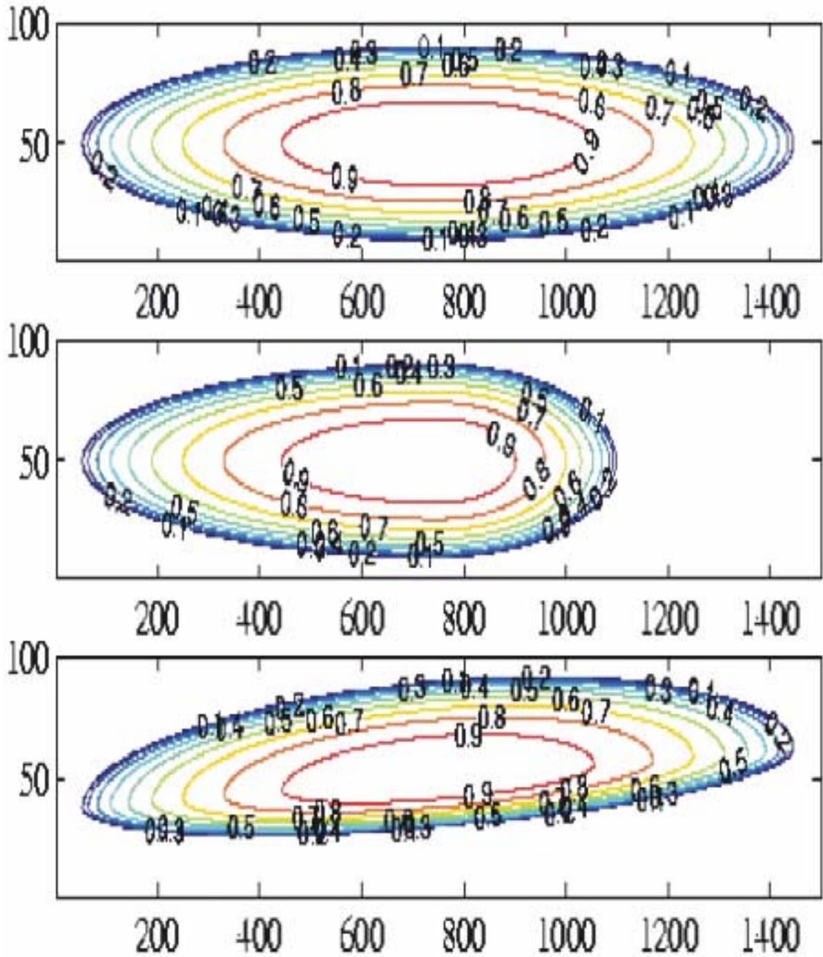
Figure 12: Example trend template ellipsoid functions to estimate sand fraction contours of the Sedflux analog.
