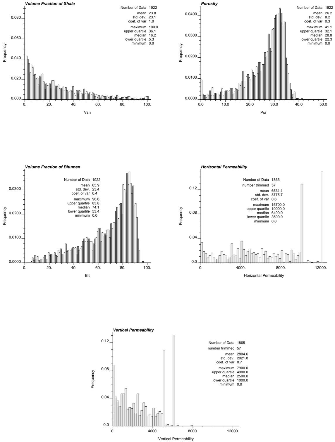
Figure 2: Histograms of the vshale, porosity, bitumen, horizontal permeability and vertical permeability.
