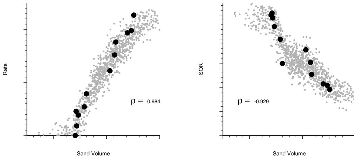
Figure 7: Relation of flow results for the twelve cases to the sand volume with filled-in synthetic values (1000 in each case). The need to *fill in* the cross plots with synthetic values is so that the production variable (rate or SOR) can be predicted for any sand volume, e.g., the sand volume at a location that has not been sampled.
