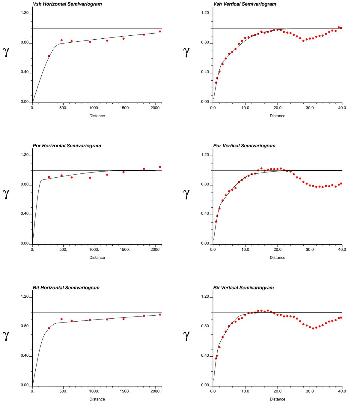
Figure 4: Horizontal and vertical variograms for vshale, porosity and bitumen.
