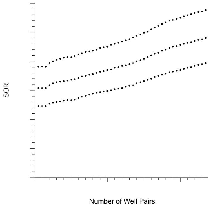
Figure 9: Average Cumulative SOR versus the number of well pairs. There are three dots for each number: the 5, 50, and 95 percentile, that is, the lowest production that could be expected, the median production expected, and the high side production. This chart relates to the *SOR* uncertainty. Note the increase in SOR for more well pairs, since lower productivity areas are produced later.
