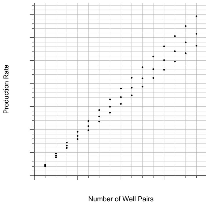
Figure 8: Cumulative production versus the number of well pairs. Note that the uncertainty increases with more well pairs and that the production does not increase linearly with the number of well pairs. This is due to the ordering of the well pairs, that is, the best locations are drilled first.
