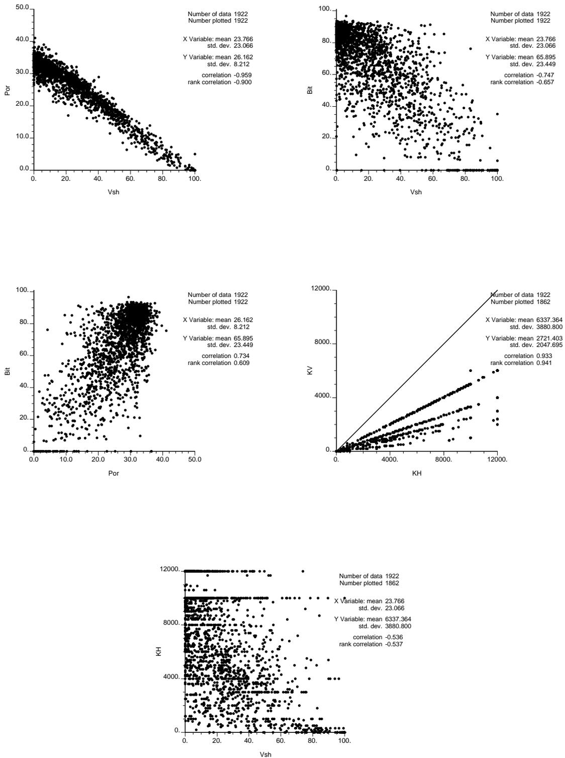
Figure 3: Scatterplots of porosity versus vshale, bitumen versus vshale, and bitumen versus porosity, horizontal versus vertical permeability, and horizontal permeability versus the volume fraction of shale.
