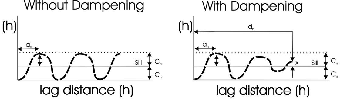
Figure 5: Parameters associated with the hole effect model
