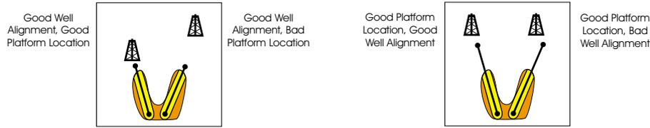
Figure 1: An illustration showing good and bad platform location and good and bad well alignment.
