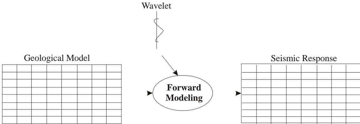
**Figure 1:** Illustration of forward seismic modeling: the geological model of acoustic impedances are read together with the Wavelet and converted to the seismic response.
