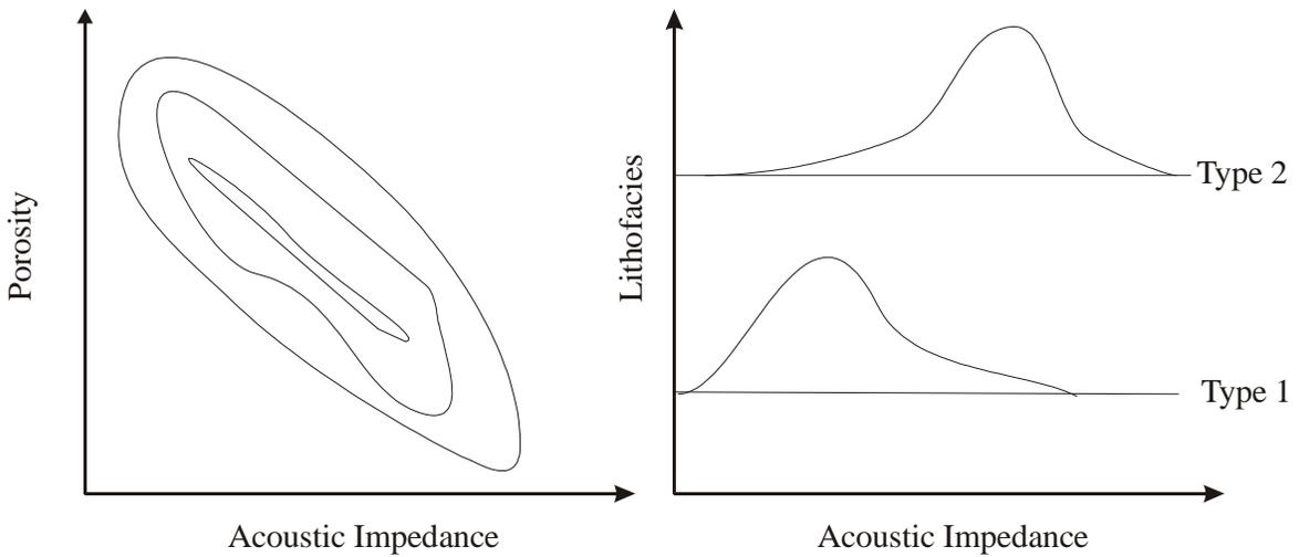
**Figure 2:** Illustration of how porosity is related to acoustic impedance (left) where the elliptical lines with negative correlation represent probability contours. The relationship between lithofacies and acoustic impedance is shown on the right, where we see a histogram of possible acoustic impedance for each lithofacies type.
