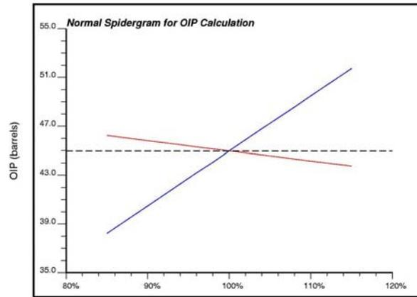
**Figure 4.2** conventional spider diagram where the change in the response variable (OIP in this case) is shown on the vertical axis relative to percentage changes in the variable. The horizontal dashed line is the base case, the blue line is porosity, and the red line is water saturation. The gross reservoir volume and the net to gross ratio would also fall on the red line because these variables go into the calculation in the same direct multiplicative manner.
