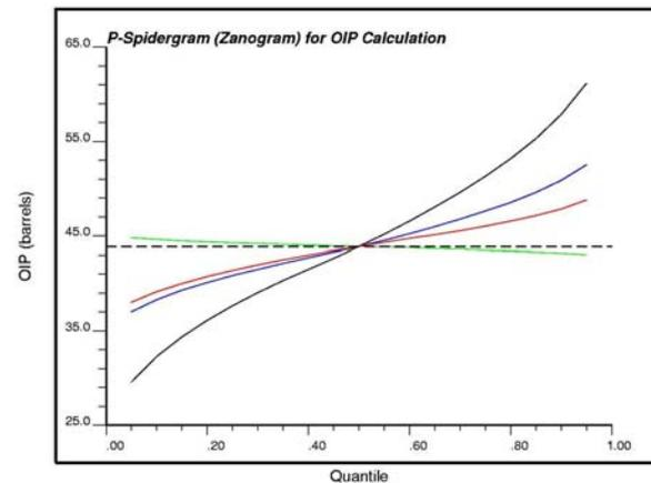
**Figure 4.3** an improved *p-spider diagram* where the change in the response variable (OIP in this case) is shown on the vertical axis relative to specific percentile values in the variable. This reflects the importance of each variable and the influence of the distribution of uncertainty. In this case the lines are: porosity (black), Sw (green), NTG (red), and GRV(blue). Note the richer information content.
