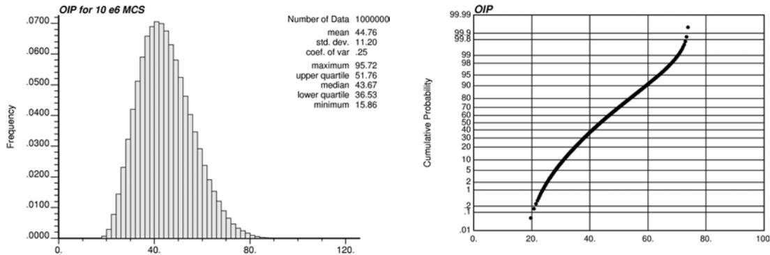
**Figure 4.1** histogram and cumulative distribution (with normal or Gaussian scale) for the oil in place for an example problem.
