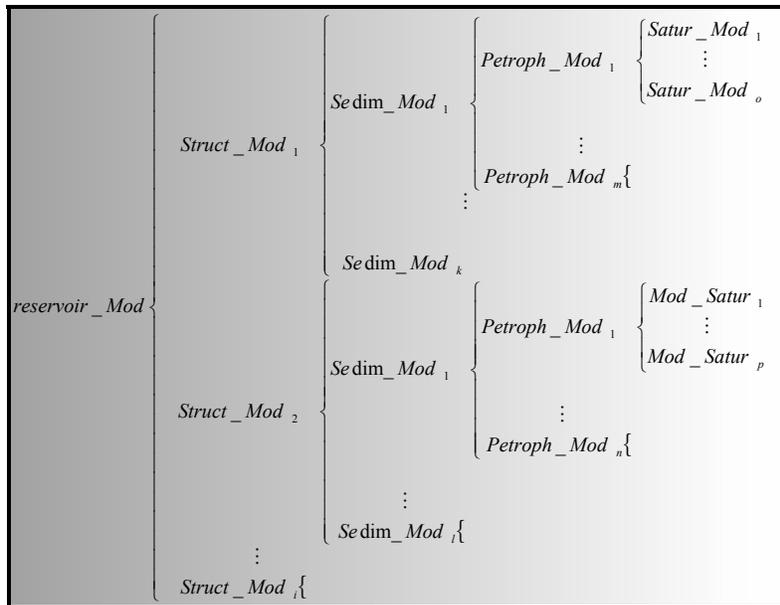
**Figure 2.5:** Scenario tree for the uncertainty assessment of a reservoir. Note that each branch has a specific number of sub-branch. For example the number of sedimentological models in the structural model 1 can be different from the number of sedimentological models in the structural model 2
