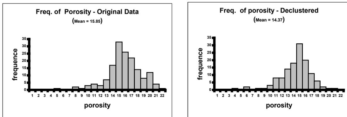
**Figure 2.1:** Equal weighted porosity histogram (left side) and histogram with declustering weights (right).
