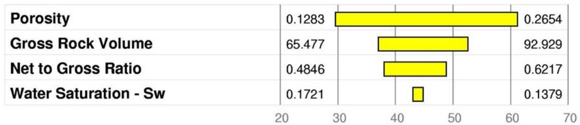
**Figure 4.4** an example tornado chart where the sources of uncertainty are explained by showing how each variable affects the final result. The numbers on the side show the P10 and P90 values that led to each result. Note that the effect of water saturation is an inverse relation.
