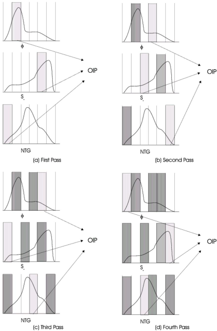
**Figure 3.2** Latin hyper cube sampling schematic illustration using three variables. (a) First pass - Random drawing from any probability interval (light grey shading); (b), (c) and (d) Subsequent passes - Random drawing from any probability interval not previously sampled. Dark grey areas are previously sampled intervals, and unavailable for future sampling. Light grey areas are the sampled interval for that particular pass.
