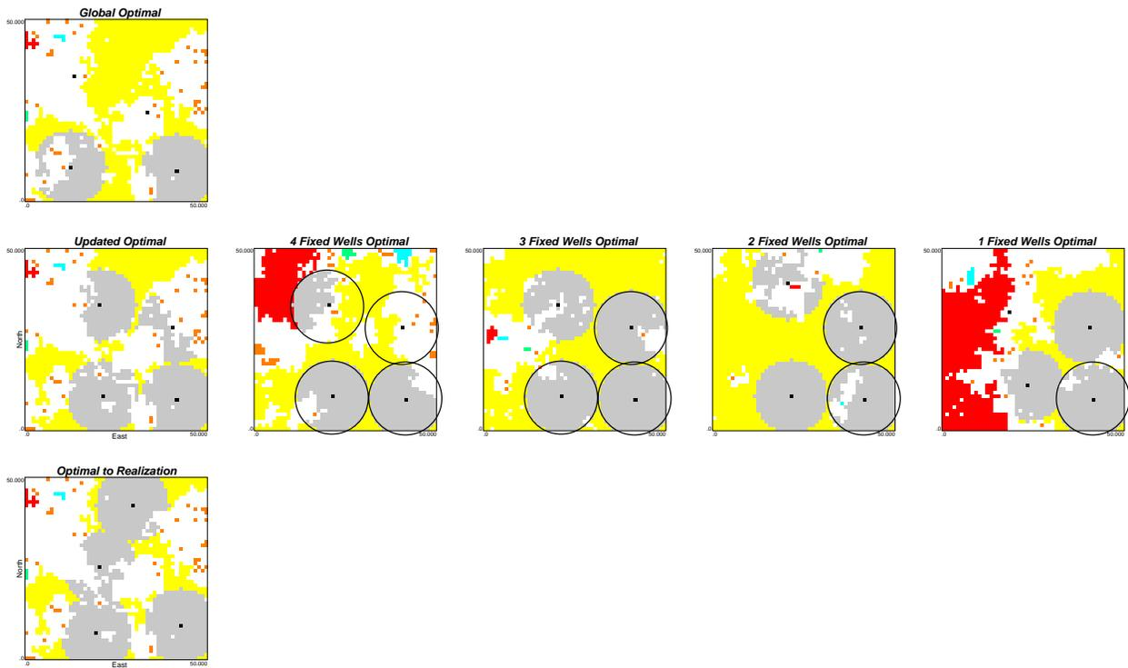
Figure 7: Together the maps represent one leg from Figure 2. The maps on the left are the geo-object maps and the placed wells for one realization for step 3, step 4d, and step 5. The maps on right from the map showing step 4c show 1 to 4 fixed wells as indicated by the heavy circles.
