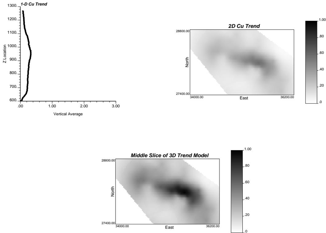
Figure 7: Required 1D trend (left) and 2D trend (middle) for integration to obtain 3D trend (right).
