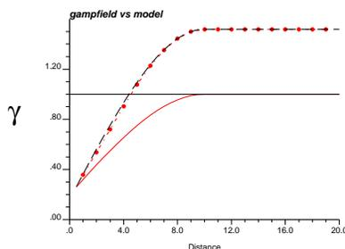
Figure 5: The calculated variogram to correct the bias generated by p-field simulation (dotted line with bullets). The original model is shown as a solid line (the sill is 1.0). The modelled variogram required to obtain unbiased realizations with PFSIM is shown as a dashed line (the sill is greater than 1.0).
