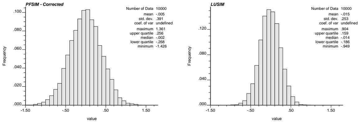
Figure 16: Histogram of the average value over the entire domain calculated from PFSIM realizations (left) and LUSIM realizations (right). Both methods reproduce the target variogram model.
