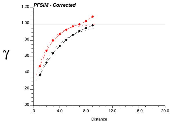
Figure 15: Unbiased variogram generated with PFSIM (dashed lines with bullets) and the target variogram model (dashed lines).
