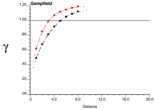
Figure 14: Corrected experimental variogram values (from GAMPFIELD) are shown as dashed lines with bullets, and model required to generate unbiased realizations (dashed lines).
