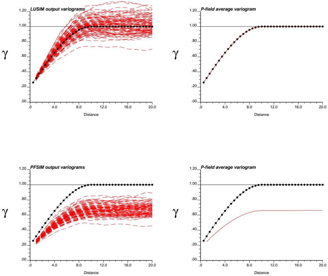
Figure 4: Performance of p-field simulation prior to correcting the variogram model to generate the p-fields. Top left: variograms of 100 LUSIM realizations used to generate the p-fields. Top right: average variogram from 1000 realizations with LUSIM. The match is perfect. Bottom left: variograms of 100 PFSIM realizations calculated with the LUSIM realizations as p-fields. Bottom right: average variogram from 1000 realizations with PFSIM. Notice the bias in variogram reproduction.
