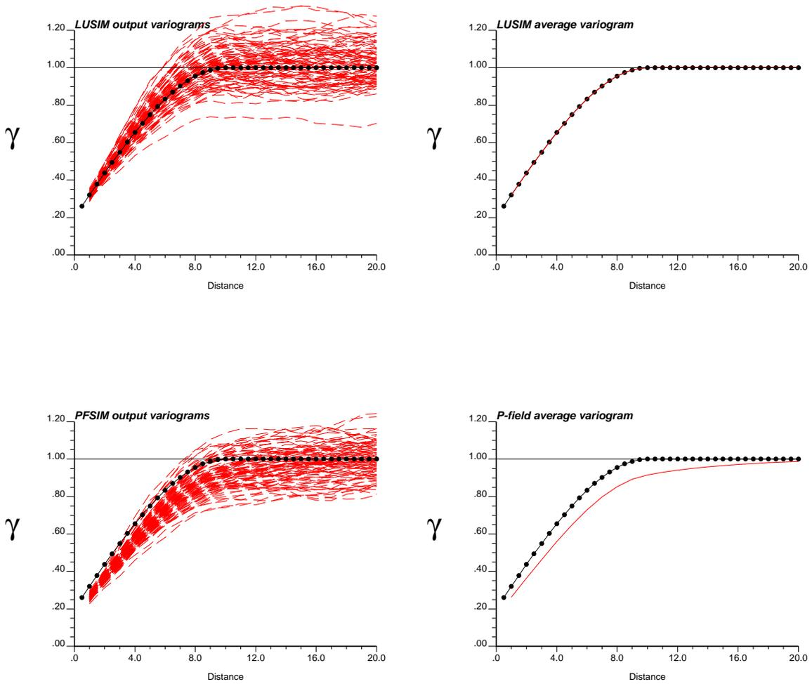
Figure 1: Performance of p-field simulation prior to correcting the variogram model to generate the p-fields. Top left: variograms of 100 LUSIM realizations used to generate the p-fields. Top right: average variogram from 1000 realizations with LUSIM. The match is perfect. Bottom left: variograms of 100 PFSIM realizations calculated with the LUSIM realizations as p-fields. Bottom right: average variogram from 1000 realizations with PFSIM. Notice the bias in variogram reproduction.
