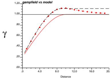
Figure 2: The calculated variogram to correct the bias generated by p-field simulation (dotted line with bullets). The original model is shown as a solid line (the sill is 1.0). The modelled variogram required to obtain unbiased realizations with PFSIM is shown as a dashed line (the sill is greater than 1.0).
