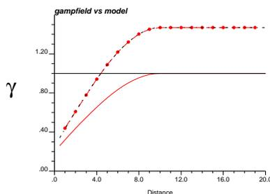
Figure 8: The calculated variogram to correct the bias generated by p-field simulation (dotted line with bullets). The original model is shown as a solid line (the sill is 1.0). The modelled variogram required to obtain unbiased realizations with PFSIM is shown as a dashed line (the sill is greater than 1.0).
