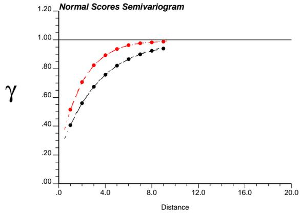
Figure 12: Target variogram model (dashed lines) and experimental variogram values (dashed lines with bullets).
