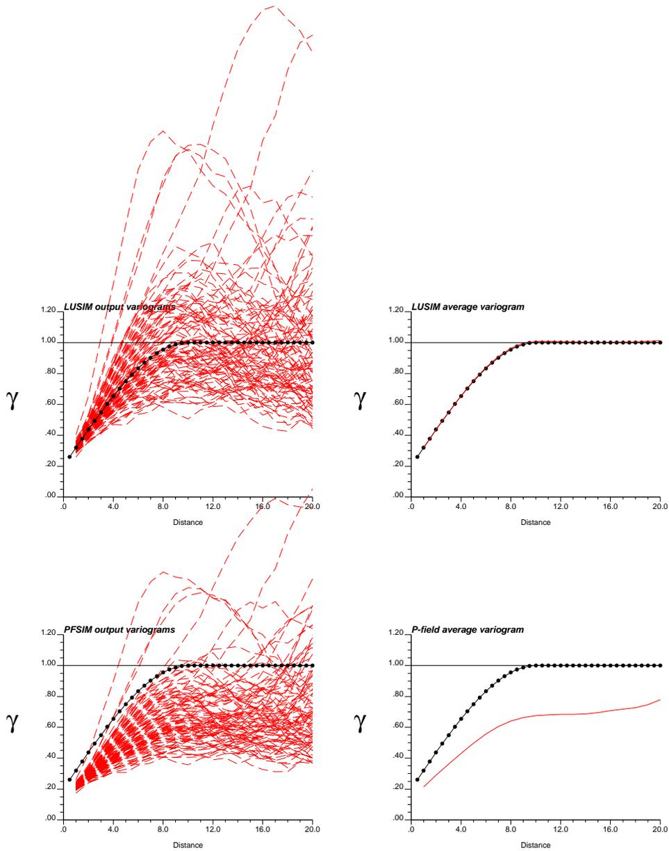
Figure 7: Performance of p-field simulation prior to correcting the variogram model to generate the p-fields. Top left: variograms of 100 LUSIM realizations used to generate the p-fields. Top right: average variogram from 1000 realizations with LUSIM. The match is perfect. Bottom left: variograms of 100 PFSIM realizations calculated with the LUSIM realizations as p-fields. Bottom right: average variogram from 1000 realizations with PFSIM. Notice the bias in variogram reproduction.
