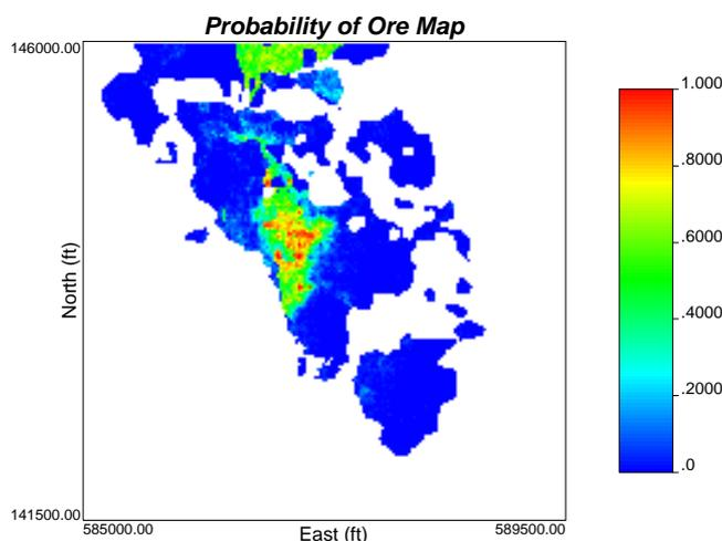
Figure 4: Probability of ore map based on stockpile criteria. The section shown corresponds to bench 850.
