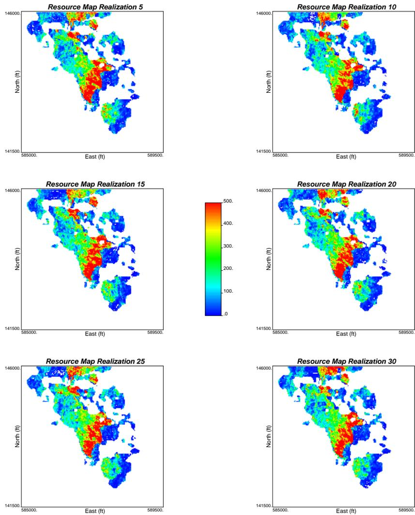
Figure 12: Six realizations of the resource models as calculated based on tonnage factors and recovery functions provided by Teck Cominco.
