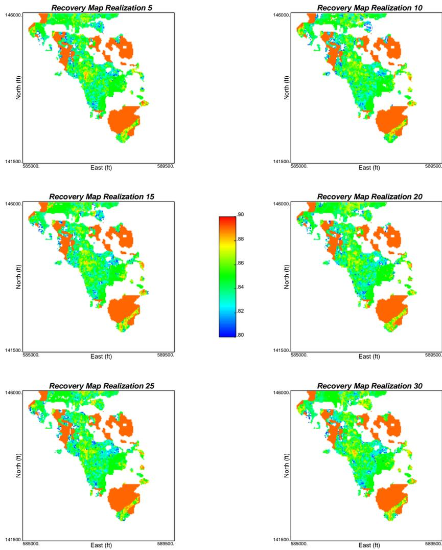
Figure 7: Six realizations of the recovery models as calculated based on recovery functions provided by Teck Cominco.
