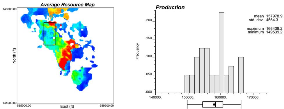
Figure 16: Illustration of application for short term planning. The volume of material associated to the planned production for one month is shown on the left, and the uncertainty in the resource available is shown on the right. The reference point plotted in the box plot of the histogram corresponds to the mean value.
