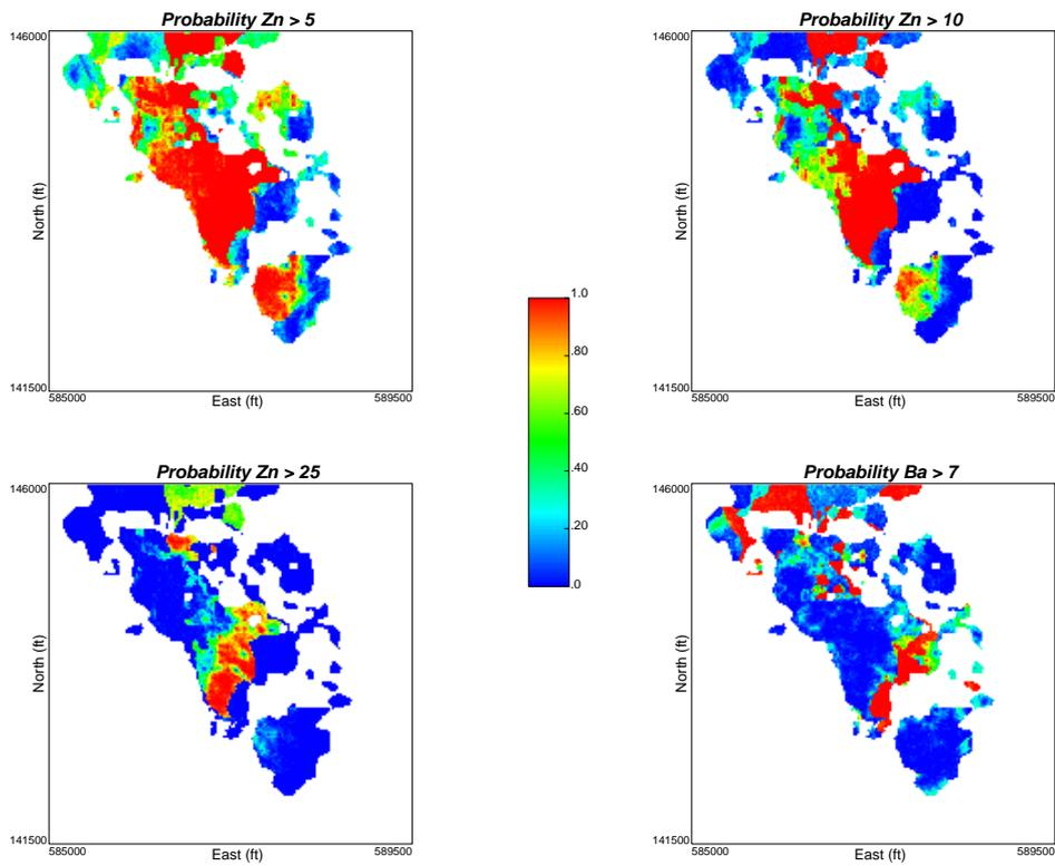
Figure 2: Probability maps to exceed a specific cutoff:  $Zn > 5\%$  (top left),  $Zn > 10\%$  (top right),  $Zn > 25\%$  (bottom left), and  $Ba > 7\%$  (bottom right). The section shown corresponds to bench 850. Note that the bottom two figures show areas of where the Zn grade is sure to be high (where the probability is close to 1.0) and the corresponding areas where the Ba grade is sure to be low (where the probability is close to 0.0).
