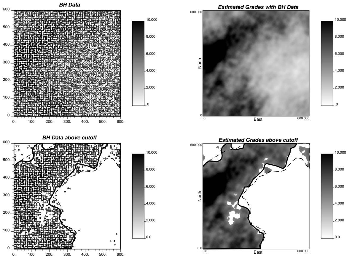
Figure 3: Maps of: (1) blasthole (BH) samples at nominally 10m x 10m spacing used for outlining ore-waste contacts (top left), (2) estimated grades based on all BH (top right), (3) only those BH samples above the cutoff grade of 5% (bottom left), and only those estimated grades above the cutoff grade (bottom right). Outline based on the estimated grades map is shown as solid line, while the outline based on BH data alone is shown as a dashed line.
