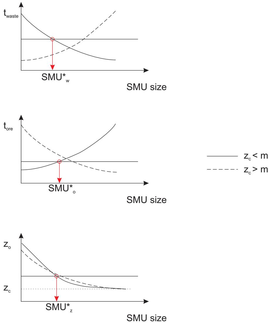
Figure 1: Schematic illustration of graphs constructed for optimal SMU size selection: tonnes of waste versus SMU size (top), tonnes of ore versus SMU size (middle), and grade of ore versus SMU size (bottom). Note that in each graph the optimal SMU size is selected for the case where the cutoff grade is below the mean grade.
