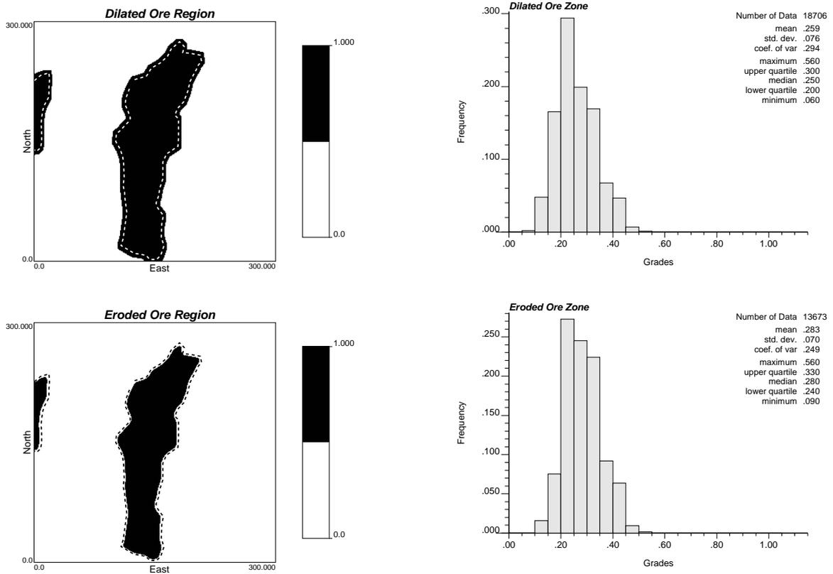
Figure 11: Example of accounting for operational dilution by (1) dilation (top) and erosion (bottom) of the original delineated ore zone. The dashed lines on the maps represent the initial ore limits.
