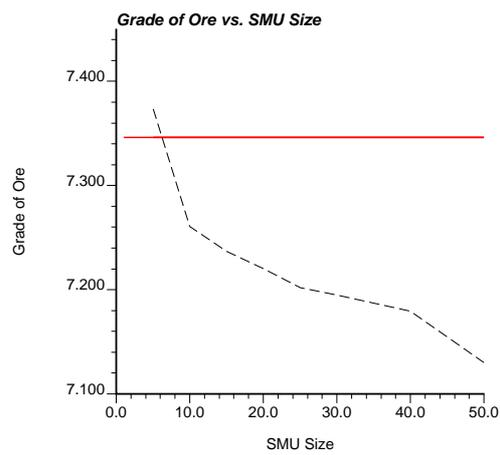
Figure 8: Graphs of tonnes of ore (top), tonnes of waste (middle), and grade of ore (bottom) versus SMU size. The reference values are plotted as solid, horizontal lines.
