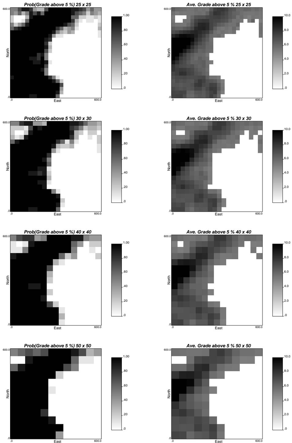
Figure 7: Probability (left) and grade (right) of ore maps for SMU sizes: 25x25, 30x30, 40x40, and 50x50.
