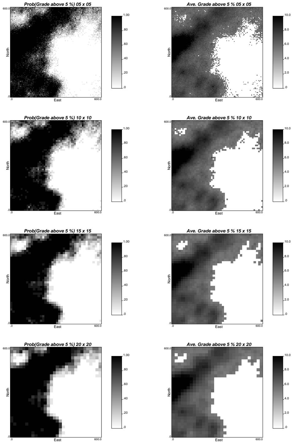
Figure 6: Probability (left) and grade (right) of ore maps for SMU sizes: 5x5, 10x10, 15x15, and 20x20.
