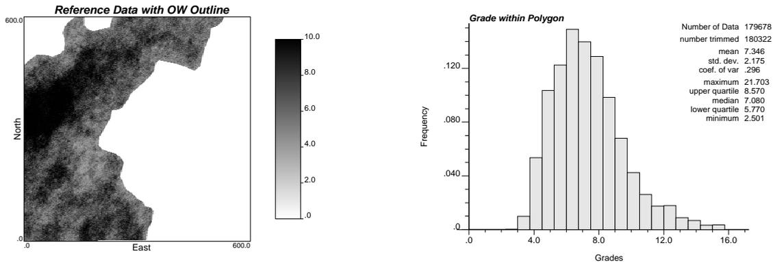
Figure 4: Map of reference grades for ore (left) and histogram of grades within the ore polygon (right).
