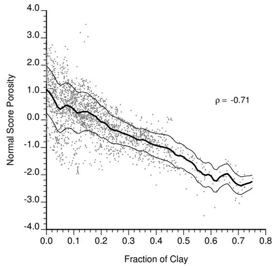
Figure 9: Scatterplot of normal score porosity versus fraction of clay with the mean porosity curve.
