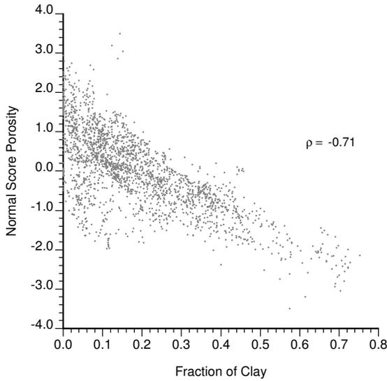
Figure 6: Scatterplot of normal score porosity versus fraction of clay.
