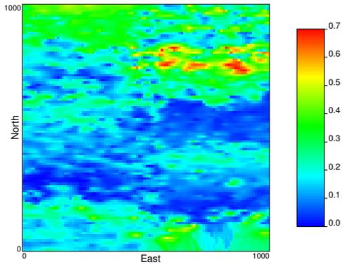
Figure 4: Fraction of clay from seismic.
