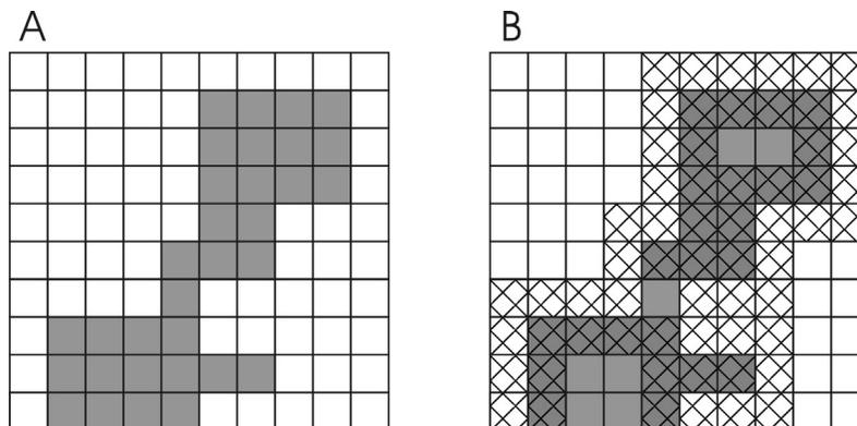
**Figure 4** – Homotopic and nonhomotopic erosions and dilations. Given the initial binomial coding (A), the locations that may be switched in the very next erosion or dilation are indicated by cross hatching.
