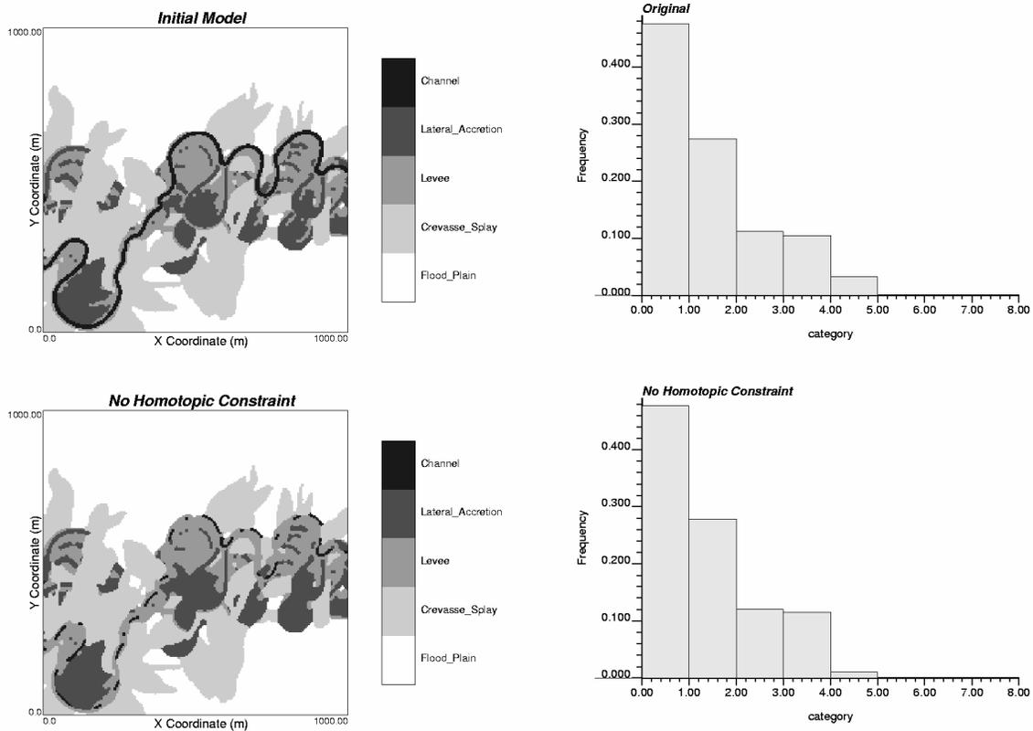
**Figure 2** – reduction in the channel fill architectural element results in discontinuous channel fills contrary to the initial model. Architectural elements: 0 = overbank fines, 1 = crevasse splays, 2 = levee, 3 = lateral accretion and 4 = abandoned channel fill.
