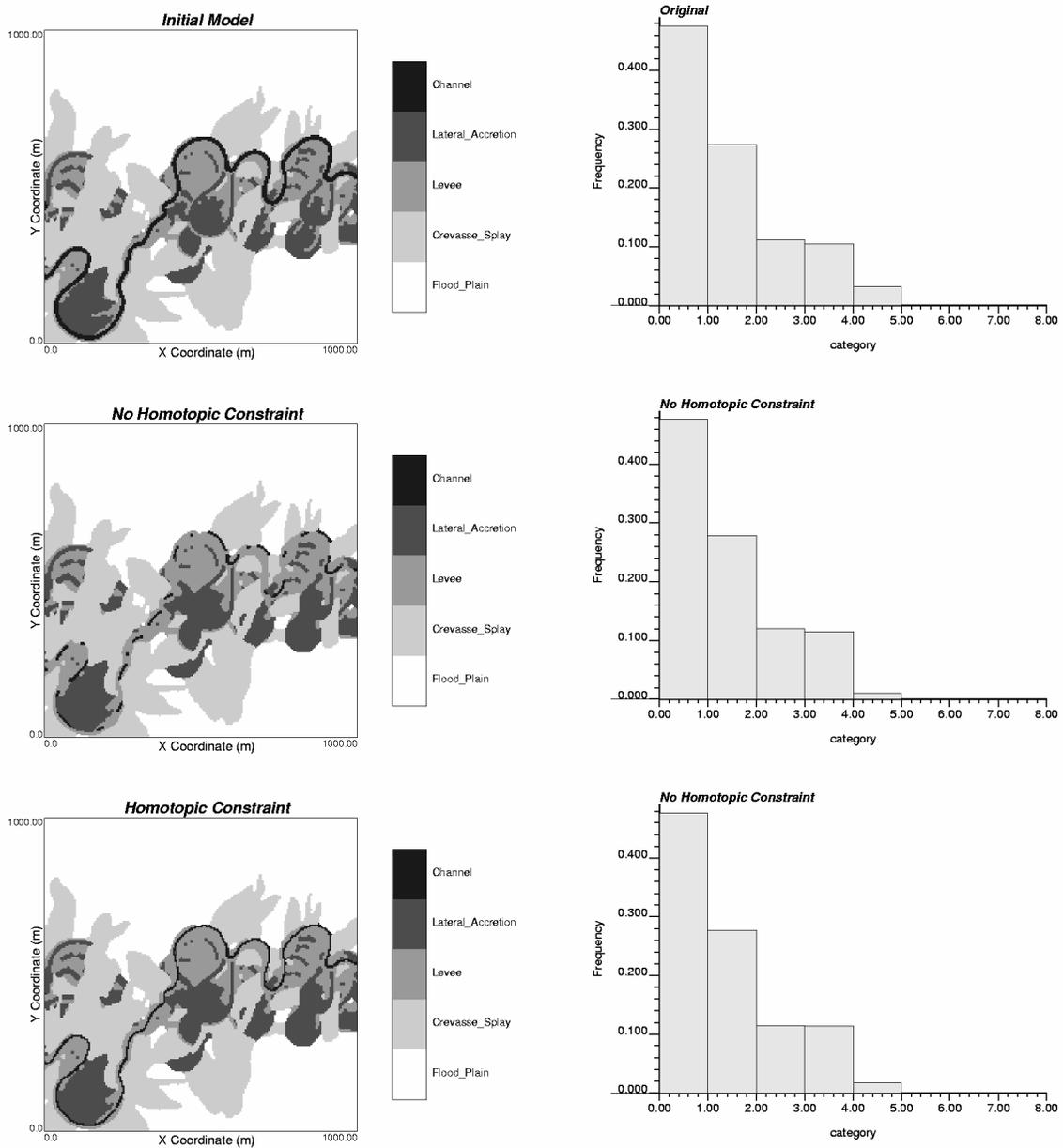
**Figure 7** – reduction in CH proportion with and without homotopic constraint on the CH architectural element alone. Architectural elements: 0 = overbank fines, 1 = crevasse splays, 2 = levee, 3 = lateral accretion and 4 = abandoned channel fill.
