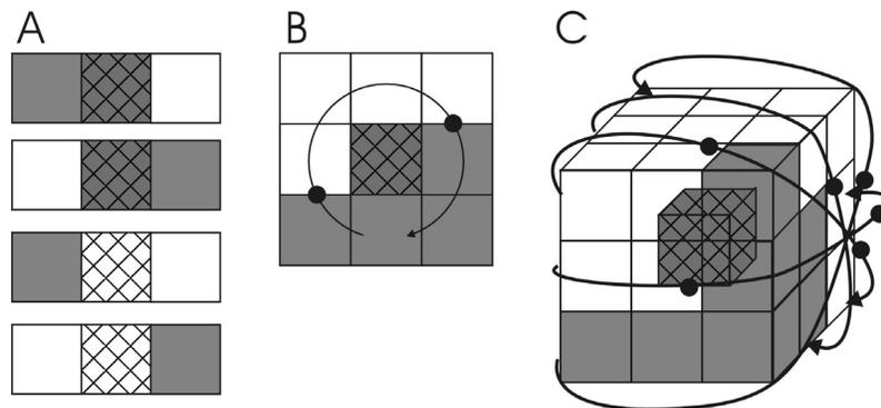
**Figure 5:** The check for homotopy of a modification. Note the hatched location is switched. A – 1-D cases that preserve homotopy. B – 2-D case for checking homotopy. If two transitions are observed over the path shown, then the switch preserves homotopy. C – 3-D homotopy is checked by applying the 2-D method in the four identified planes. Transitions are identified by black circles.
