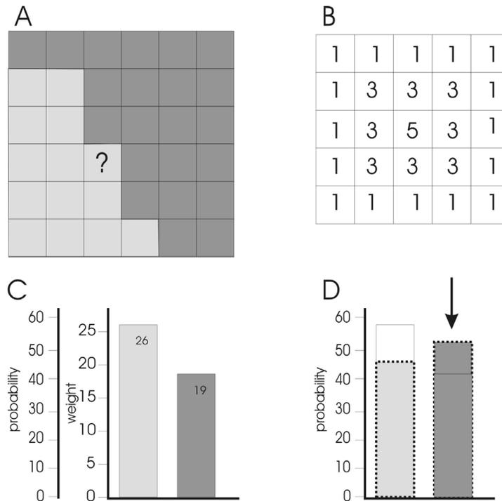
**Figure 1** – the MAPS algorithm. Given a 2-D model with two categories (A) and a weight template (B) the probability (%) of each category is calculated (C). The probabilities are scaled by factors (target proportion divided by the proportion after the last iteration) to improve reproduction of the global pdf (D). The category with the maximum probability is selected (indicated by the arrow).
