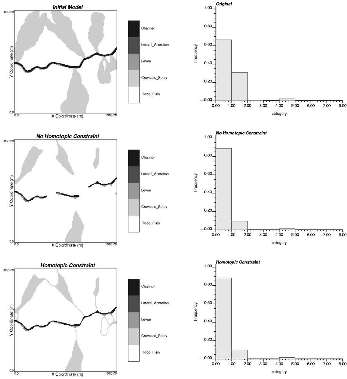
**Figure 8** – reduction of channel and crevasse splay proportions with and without a homotopic constraint on the architectural element group (CH, LV and CS). Architectural elements: 0 = overbank fines, 1 = crevasse splays, 2 = levee, 3 = lateral accretion and 4 = abandoned channel fill.
