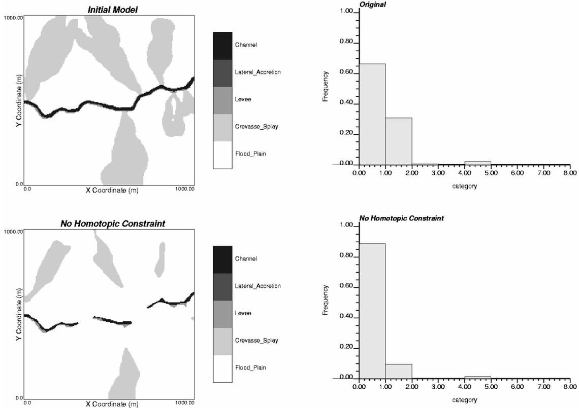
**Figure 3** – Reduction in the channel fill, levee and crevasse splay architectural elements results in distortion of expected connectivity relationships. Architectural elements: 0 = overbank fines, 1 = crevasse splays, 2 = levee, 3 = lateral accretion and 4 = abandoned channel fill.
