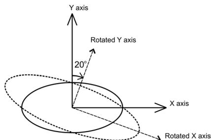
**Figure 1:** Rotation to capture the true anisotropy. The solid lines are the original coordinate system and the apparent anisotropy. The dashed lines are the rotated coordinate system and the true anisotropy.
