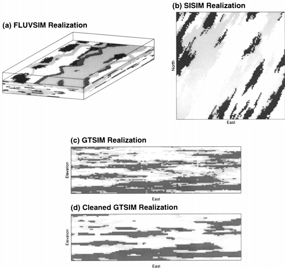
Fig. 7. Examples of facies modelling: (a) isometric view (generated with *isoview*) of *fluvsim* object-based facies model, (b) horizontal slice through *sisim* indicator simulation, (c) cross-section through facies model created by truncated Gaussian, *gtsim*, technique and (d) cross-section through realization after 'cleaning' with maps.
