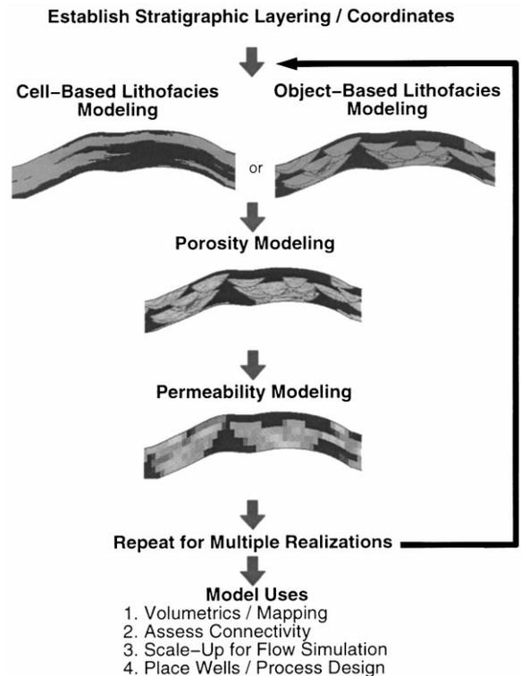
Fig. 1. High-level geostatistical reservoir-modeling flow chart: the structure and stratigraphy of each reservoir layer must be established, lithofacies modeled within each layer, and then porosity and permeability modeled within each lithofacies.
