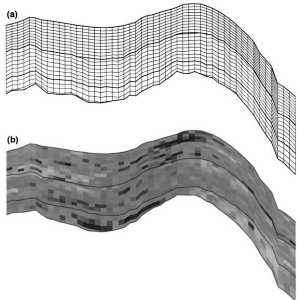
Fig. 4. Example output from `secview`: (a) gridding scheme—note ‘erosion’ at top of middle layer and ‘onlap’ at the bottom of bottom layer and (b) color coded according to petrophysical property such as porosity.
