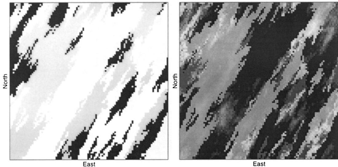
Fig. 8. Facies model and corresponding porosity model. Porosity values in each facies type were generated independently with `sgsim` program.
