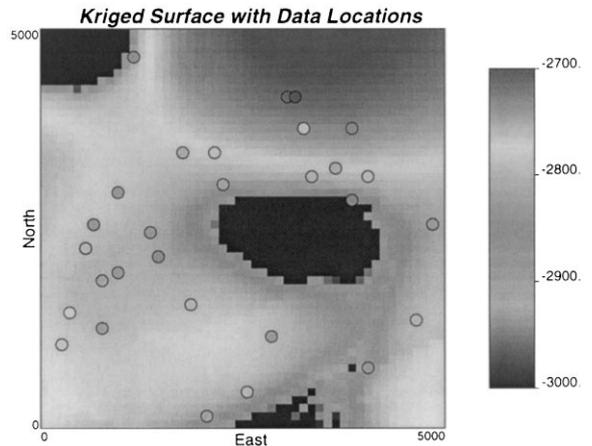
Fig. 3. Color scale map of kriged structural surface with well locations posted on map. Created by combining PostScript output of `pixelplt` and `locmap`. Negative kriging weights make it possible to estimate surface at lower elevations than smallest data value.
