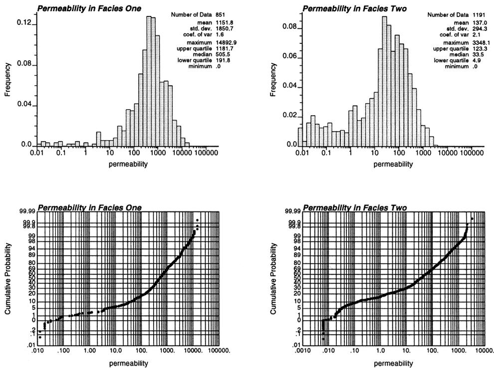
Fig. 5. Example histograms and probability plots for two facies types within same reservoir layer.
