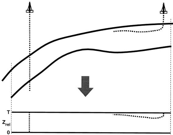
Fig. 2. Illustration of  $z_{rel}$  coordinate calculation for proportional stratigraphic correlation.
