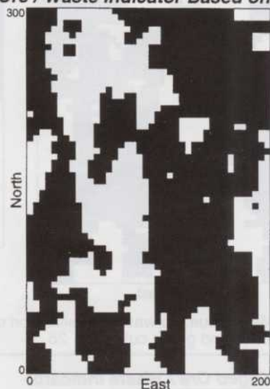
Figure 12 — Map of ore/waste classification based on maximum profit selection.
