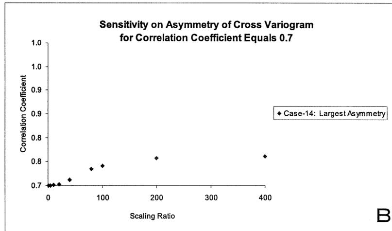
**Figure 7.** Sensitivity runs for cross-variogram asymmetry to illustrate effects of equal contribution, partial, and large asymmetry. A, Sensitivity on asymmetry of cross variogram to illustrate effect of partial asymmetry. Correlation coefficient fixed to 0.7 for cross variogram; B, Sensitivity on asymmetry of cross variogram to illustrate effect of largest asymmetry. Correlation coefficient fixed to 0.7 for cross variogram.
