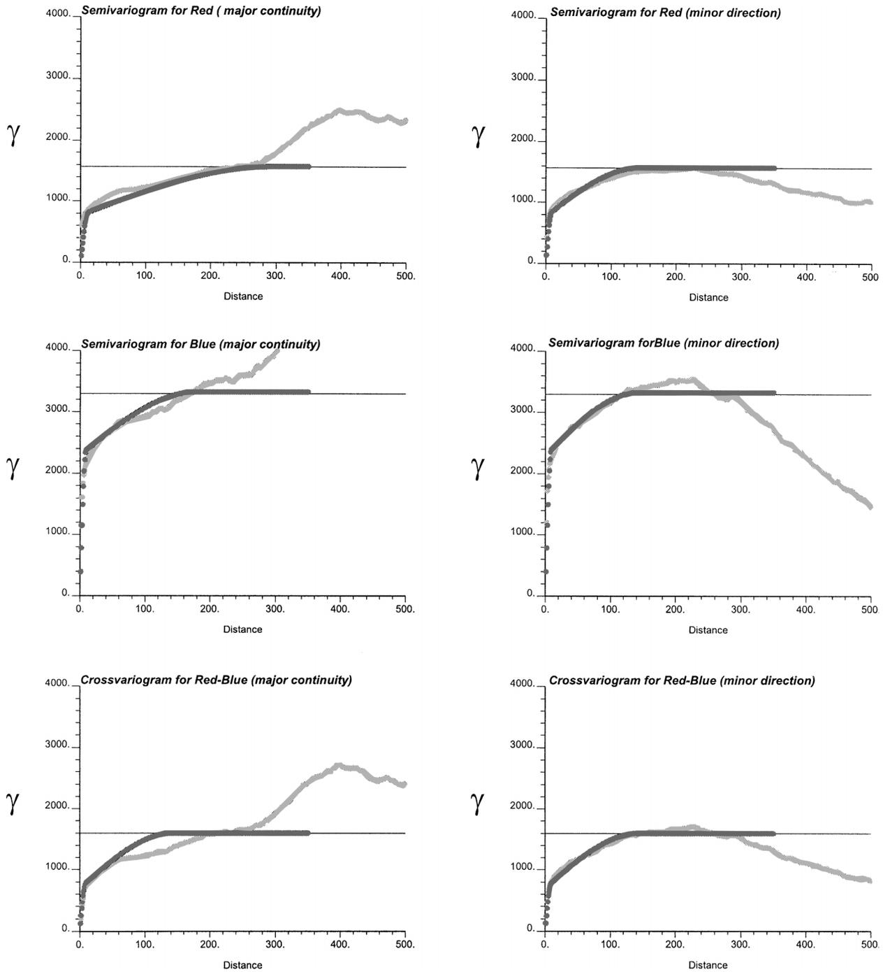
Figure 9. Experimental directional direct and cross variograms for “red” and “blue” data along with fitted LMC model.
