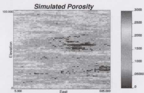
Fig. 12. Color scale image of simulated porosity. This is a vertical cross section. The two vertical wells are at either end of the cross section.
