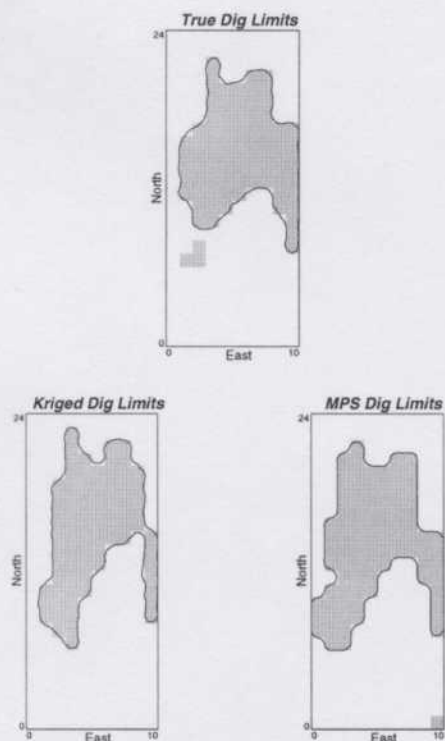
Figure 8: The converged dig limits for the true, kriged, and MPS ore - waste maps.
